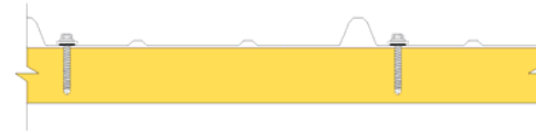
Fig. 3 We use 29ga. Grade E steel, ribbed 9" on center, with the industry leading Kynar500 40 year paint system. All steel is fastened with stainless-steel Buildex® Screws for maximum holding power.
